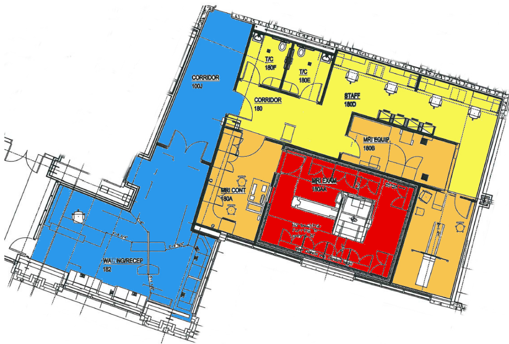
Fig. 1. Blueprint of CB3 MRI Facility. Zones are color coded. Zones 2-4 are referred to as the MRI Suite.
